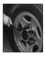
If your vehicle has wheel nut caps, loosen them by turning the wheel wrench counterclockwise. If the vehicle has a center cap with wheel nut caps, the wheel nut caps are designed to stay with the center cap after they are loosened. Remove the entire center cap.
